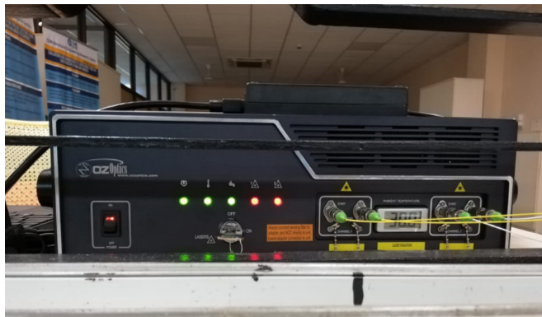
Fig.1 Distributed strain and temperature measurement system
